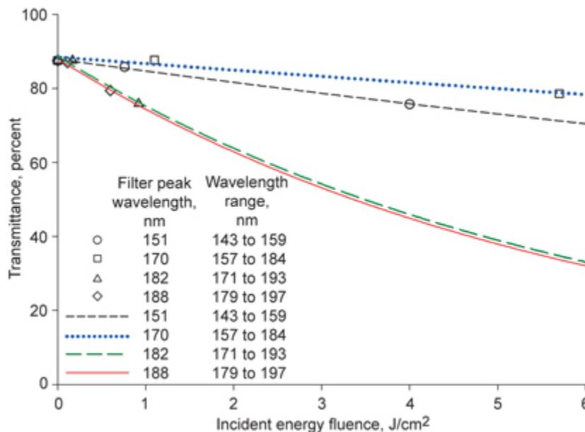
Figure 8. Transmittance of 152-µm DC93-500 silicone film at 250 nm as a function of incident VUV energy fluence provided by exposure to various wavelength ranges through
