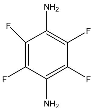
Figure 3. Chemical structure of para- 4F Diamine
